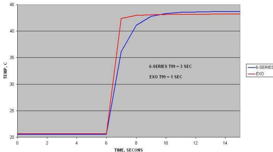
Figure 1: Comparison of response time between EXO and 6-Series temperature sensors. Transfer from ambient temperature water to hot water with rapid stirring.
