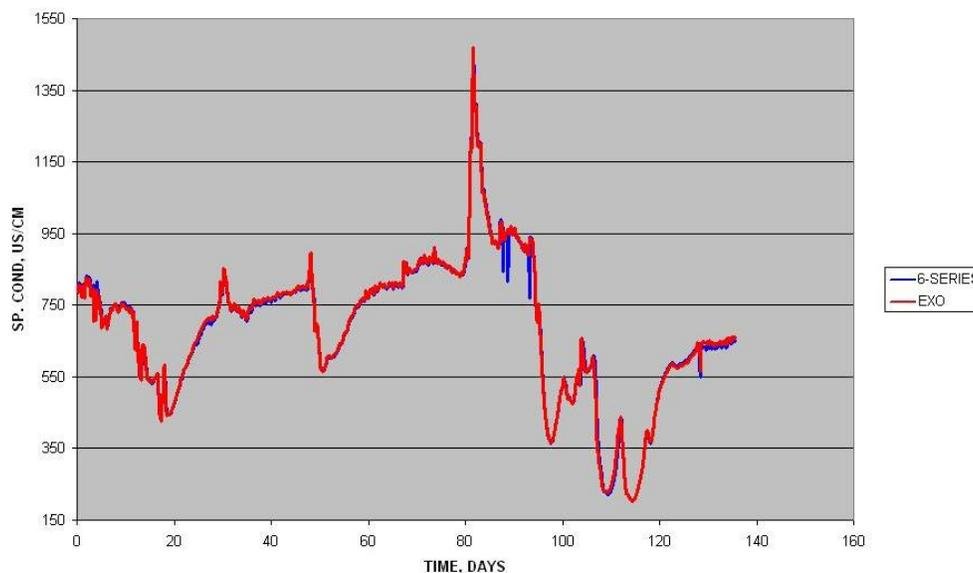
Figure 2: Comparison of specific conductance between EXO and 6-Series in Miami River, OH over 140 days.
