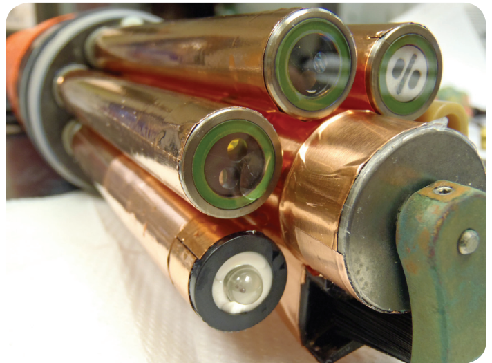
An EXO sonde prepped for deployment with anti-fouling copper tape.
